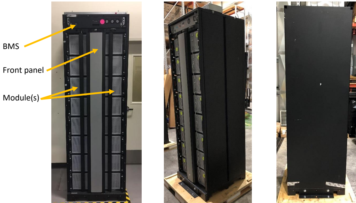
Figure 3-3: Photos of NMC rack; front (right), side (middle), and back (right).
