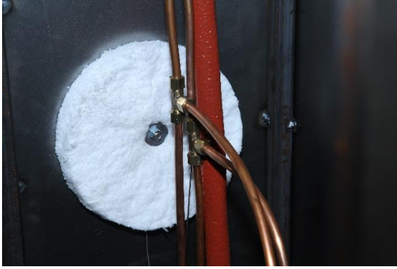
Figure 3-8: Photo of backside of TCs installed on mock ESS rack (TC28 – 37) on left and schematic of TC attachment on right.
