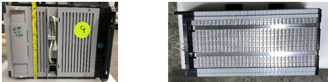
Figure 3-4: Photos of NMC module; front face (left) and top with front face of module shown on left side of picture (right)
