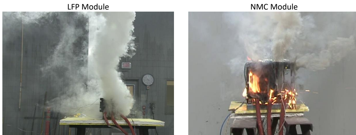
Figure 4-6: Example of LFP (left) and NMC (right) battery response to abuse conditions. LFP batteries vented a thick white smoke and sometime required an external pilot flame to ignite, whereas NMC batteries generate sparks that consistently ignited vent gases.
