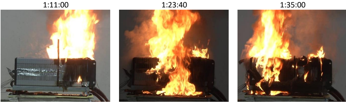
Figure 4-7: Side view of lateral fire propagation for NMC module; in this view the ignition heaters are located on the right half (front) of the module and the fire progress from the right to left.
