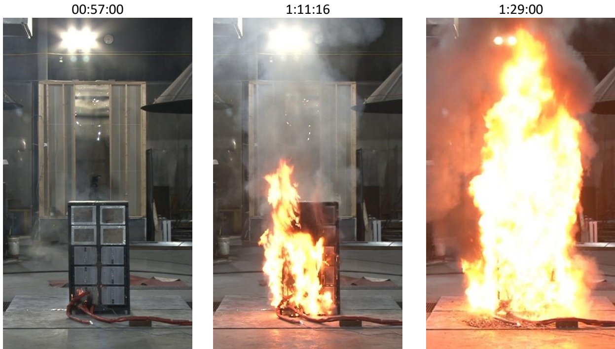
Figure 5-5: Photos of NMC fire development during intermediate-scale free burn test: near time of ignition (left), near time of predicted sprinkler operation (middle), peak heat release rate (right).
